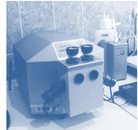
Fig.1. A – graph of skeletal muscle respiration (oxygen concentration, blue line; respiration rate, red line), B – graph of mtMP (mtMP, black line; mtMP dynamics, green line), C – Oroboros O2k-Respirometer (Oroboros Instruments, Austria)
